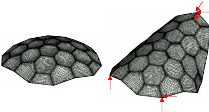
*Fig.3 Deformed plot of two identical, but differently supported, faceted shell structures loaded by the same vertical load. The scale difference between the two plots is 4500.*
