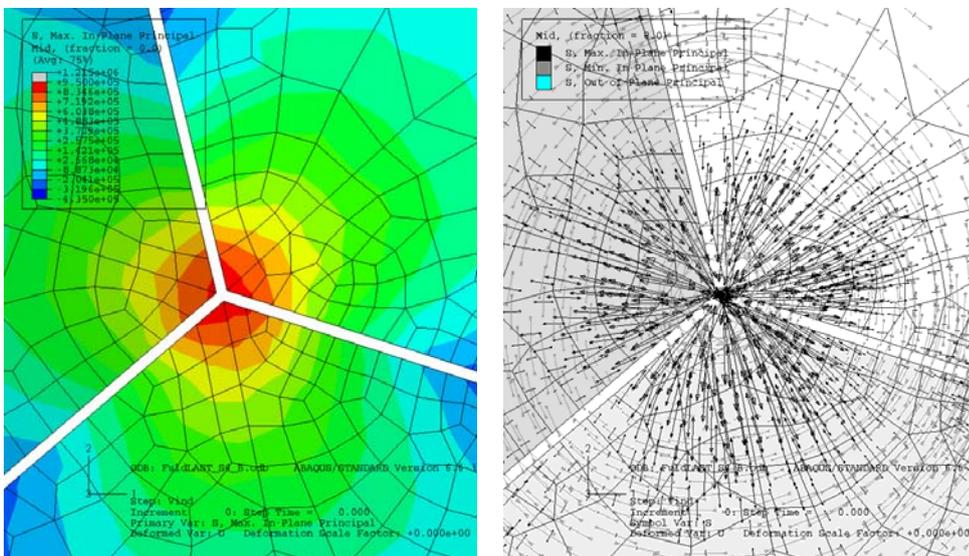
Fig.4 Membrane stresses in a vertex of the faceted shell, for a uniformly distributed vertical load of 0.72 kN/m<sup>2</sup>. The glass plate thickness is 10 mm. The calculated structure is described in section 5.
