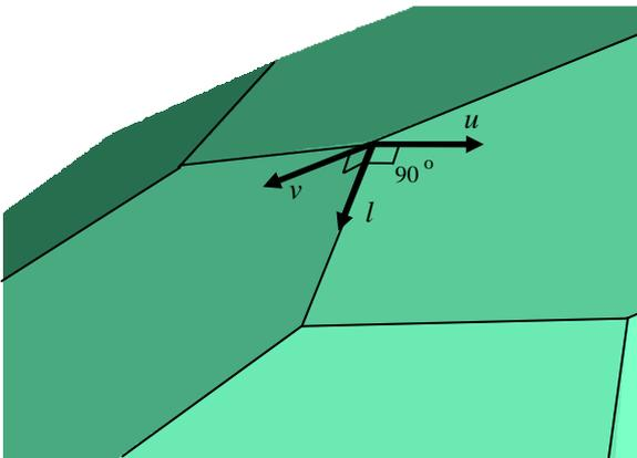
Fig.5 A connection line in a plane-based faceted shell structure.
