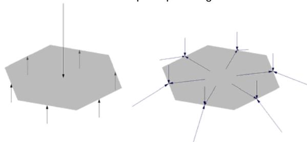
*Fig.2 Principle sketch of local bending action in a facet, and resolving of the out-of-plane reaction forces into in-plane stresses at the facet edges.*
