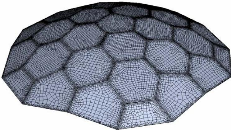
*Fig.1 Finite element model of faceted shell structure.*
