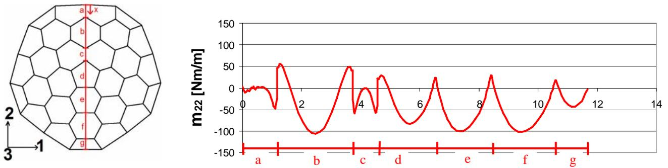
Fig. 7 Bending moment  $m_{22}$  along the indicated line across the structure for uniform snow load. A bending moment of  $100\text{Nm/m}$  corresponds to a tension of  $6\text{MPa}$  in the glass surface from bending.
