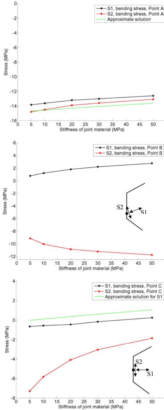
Figure 4: Bending stress in the three evaluated points. Analysis series 1.
