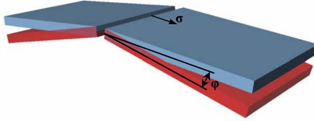
Figure 1: Rotation in joint. The red plate illustrates the deformed facet.
