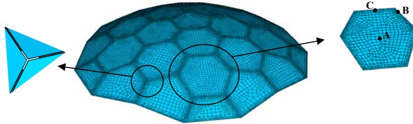
Figure 3: Faceted glass shell modelled in Abaqus. The image to the left shows the detail in the corner, where a much more flexible material replace the stiff joint along the first 10cm from the glass corner.
