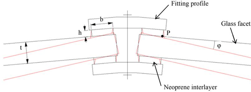
Figure 2: Connection design. The stiffness of the fitting profile is large compared the neoprene.
