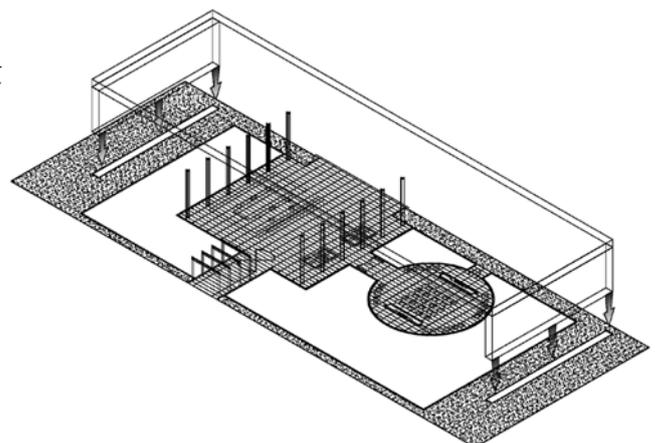
structure. Circular glass columns were initially considered but the design was eventually fixed on cruciform glass columns made up from multiple-layer laminated glass.
