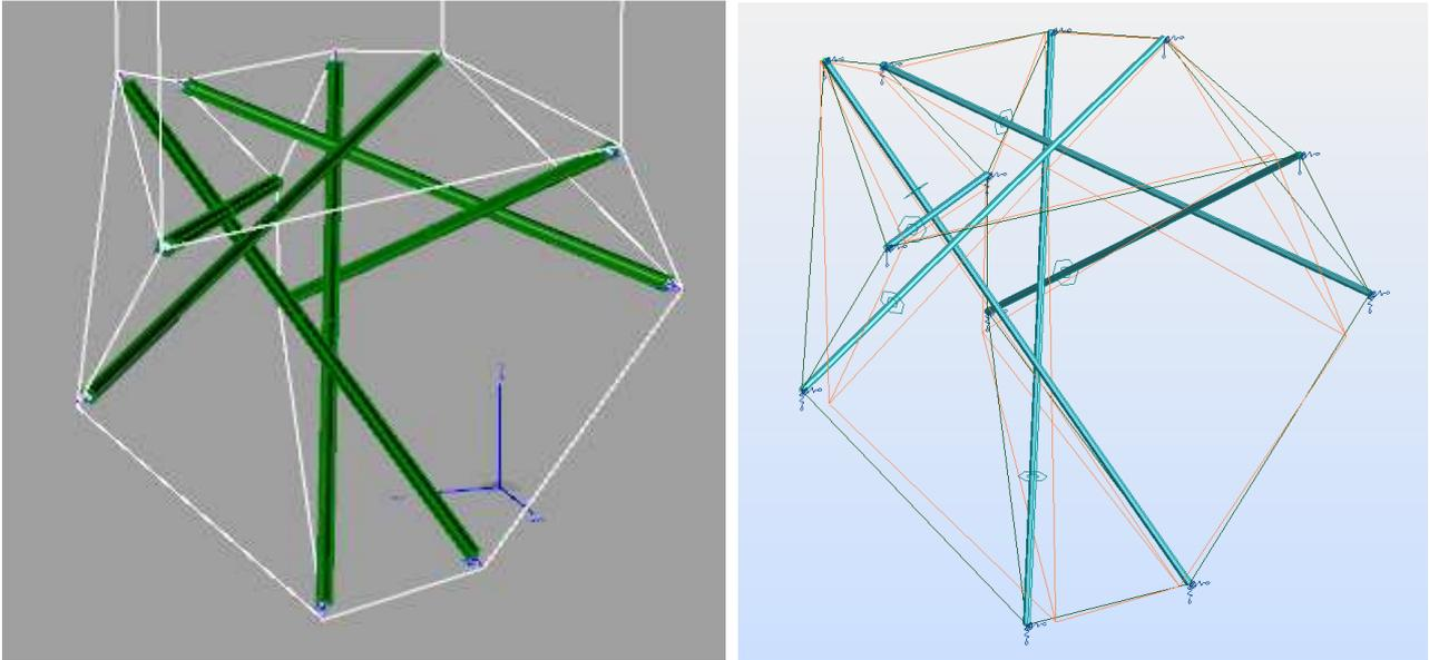
Figure 4: The revised model (above) and its deflected shape (below).
