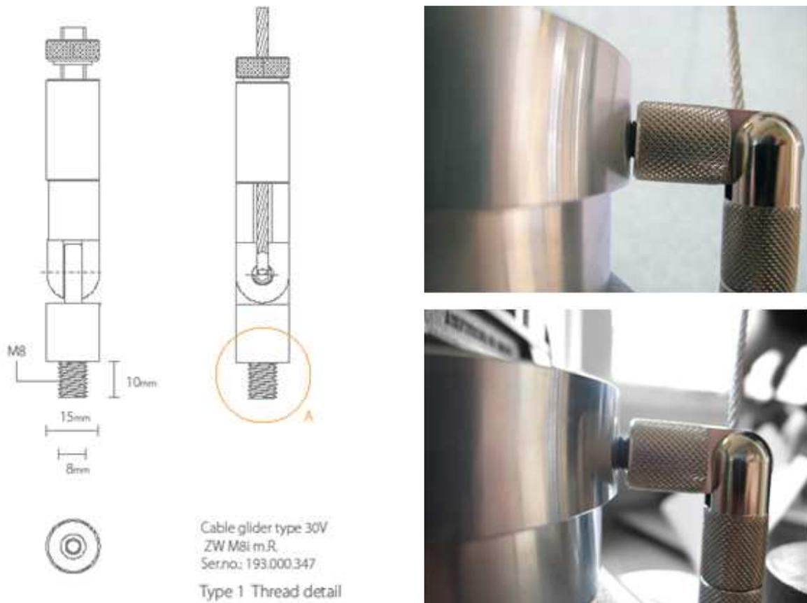
Figure 6: Grip-glider drawing (left) and Load testing of the screw-end for bending and deflection (right)
