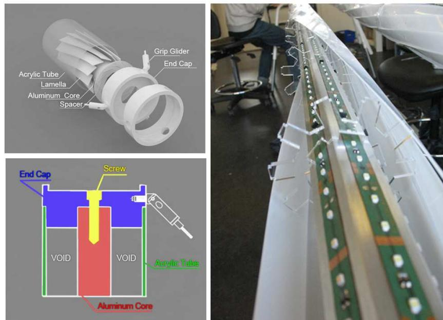
Figure 5: Assembly of a compression member (left top and right), a drawing of an end-cap (left bottom)
