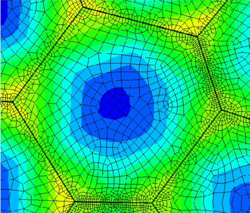
**Figure 7.** Result of the described FE-calculation. Largest in-plane principle stress in the upper side of the shell elements. The definite value of the stresses is not shown. The stress distribution does not imply moment singularities near the plate corners.
