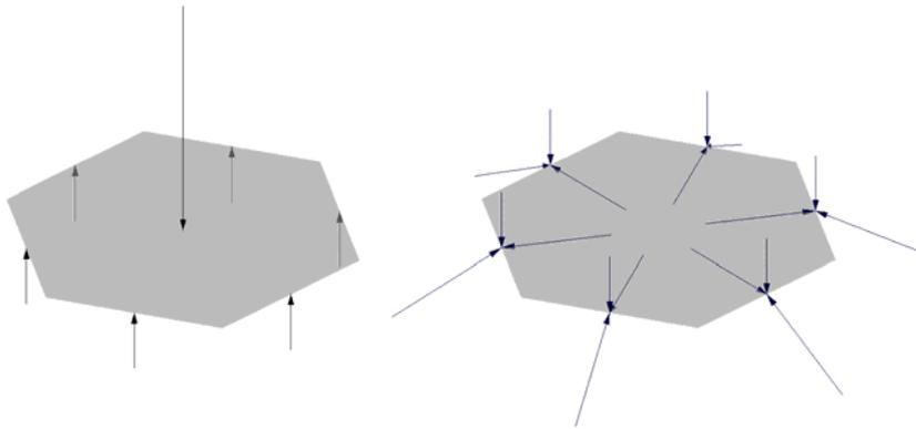
**Figure 4.** Local bending action in a facet, and decomposing of out-of-plane forces into in-plane stresses at the facet edges.
