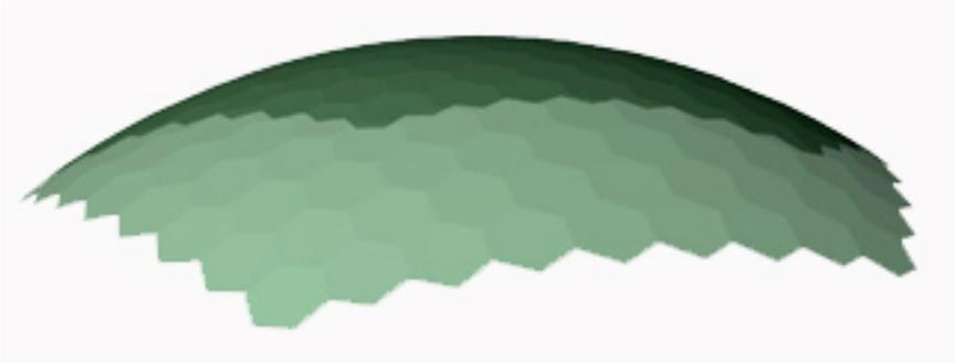
**Figure 6.** Rendering of glass dome with three-way vertices.
