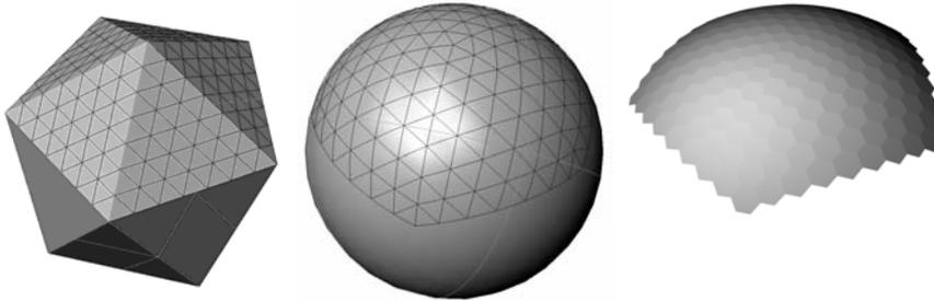
**Figure 2.** How to construct a Geodesic sphere from an icosahedron. The image to the right shows the plane based dual to the triangulated geometry in the centre image.
