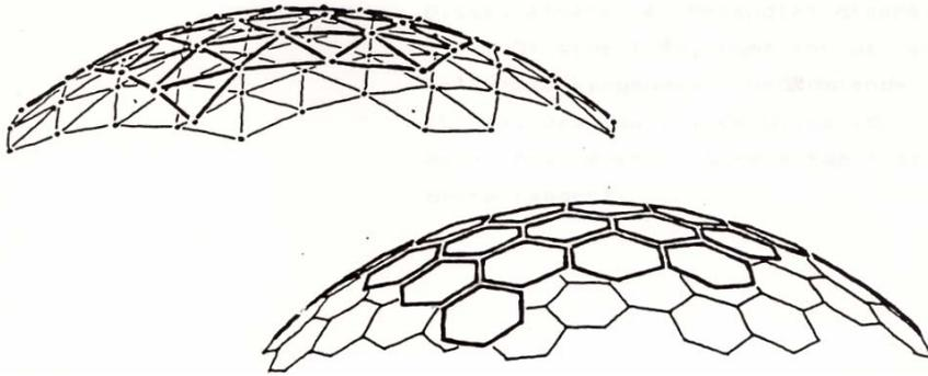
**Figure 3.** Two dual shells structures, with triangular facets and three-way vertices respectively.
