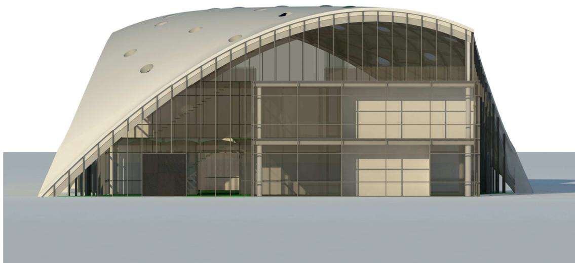
Fig. 1: Super-light student project with ribbed shell and Pi-Omega system. By Andreas Castberg.
